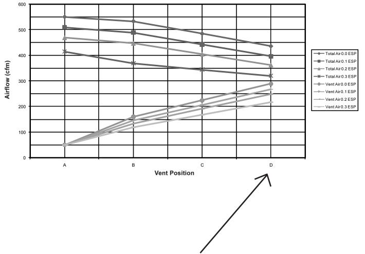
Brown/white wire must be switched from terminal X to terminal D on damper motor to attain "D" position. This will bypass potentiometer function and go to "full open" when energized.
